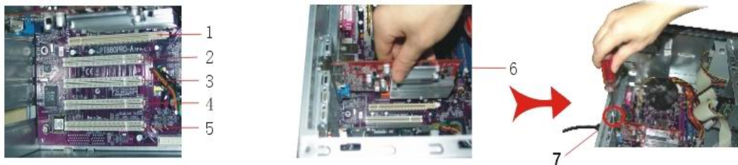
(1. Display Card slot; 2-5 Slots for Sending Card and TV or Video Capture Card; 6 Display Card; 7 Reinforcement Screw for Display Card)
