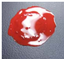
Counter Sunk Screw head coated with “Corona Dope”
