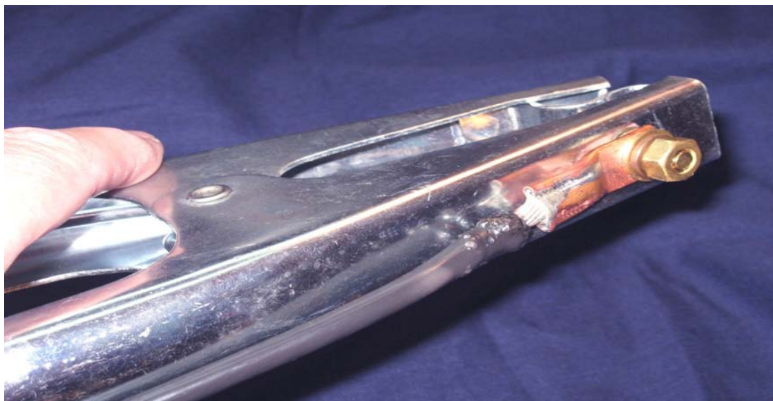
A welding clamp is a handy device for connecting the RF Ground
