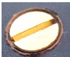
Counter Sunk Screw head coated with “Corona Dope”
