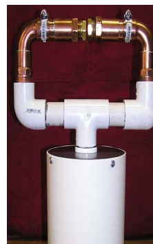
“Sucker Gap” (vacuum in the base for quenching)
