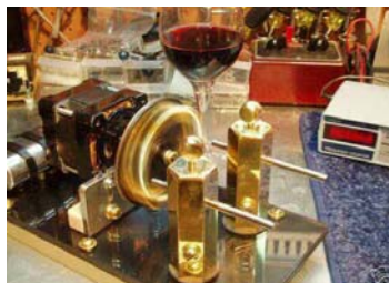
Synchronous Rotary Spark Gap
