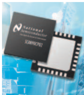
The 1.5-Gbps, 2×2 Scan90CP02 LVDS crosspoint switch has programmable pre-emphasis and support for IEEE 1149.6 to enable testing of ac-coupled interconnects.
