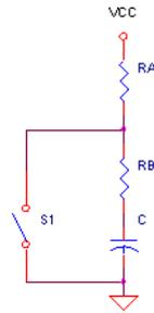
**Switch OFF → Charge C, Switch ON → Discharge C.**
