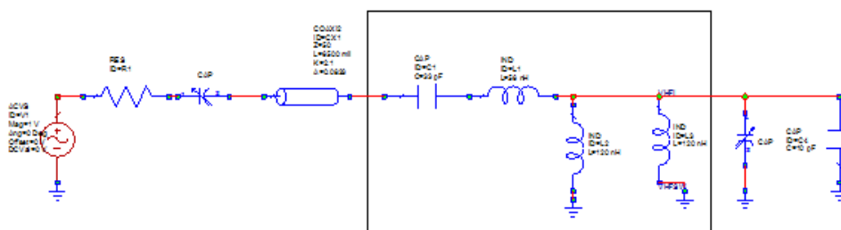
Figure 18. Silicon Labs Recommended FE Network
