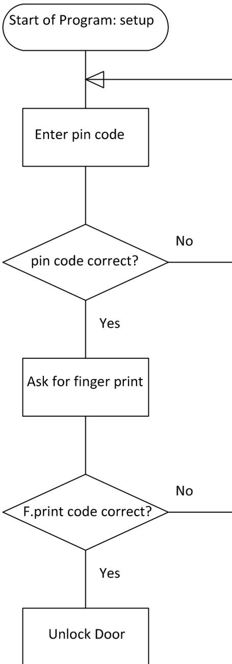
A pin code is entered on the keypad, this pincode will open a memory/register which contain the fingerprint data.
