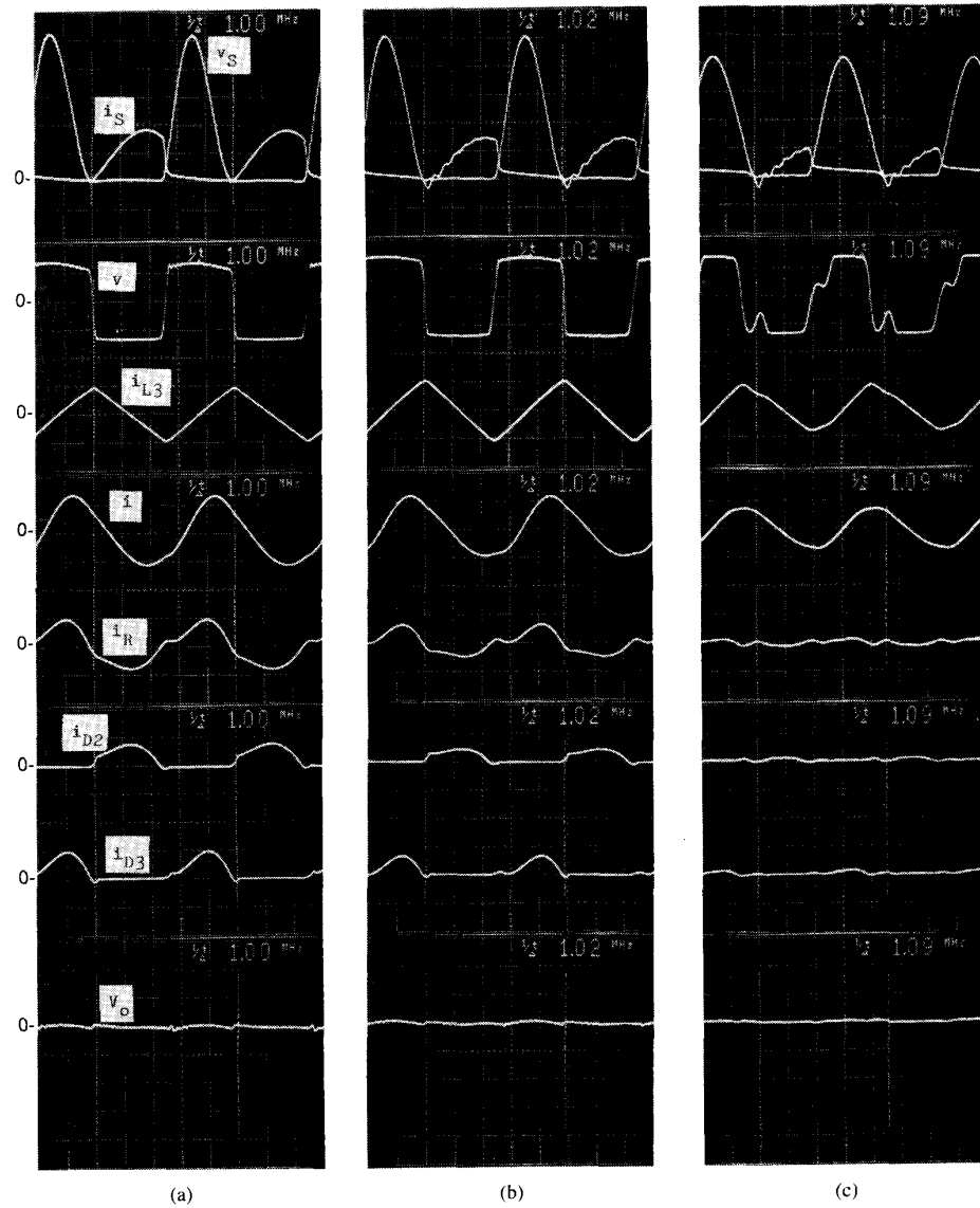
Fig. 7. Experimental current and voltage waveforms in converter of Fig. 6(a). (a) For optimum operation ( R_L = 200 \Omega ). (b) For continuous mode of operation ( R_L = 300 \Omega ). (c) For discontinuous mode of operation ( R_L = 3 \text{ k}\Omega ). Vertical: 1 A/div. for all currents, 20 V/div. for v_s and v , and 1 V/div. for ac component of V_o ; horizontal: 200 ns/div.
