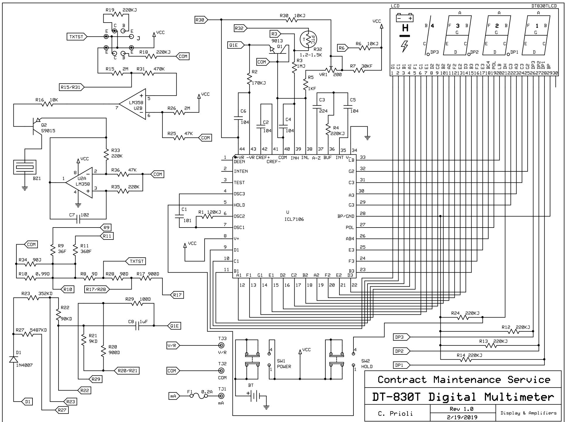
P:\DT-830T Digital Multimeter\DT-830T Digital Multimeter Schematic.sch - Main Circuits
