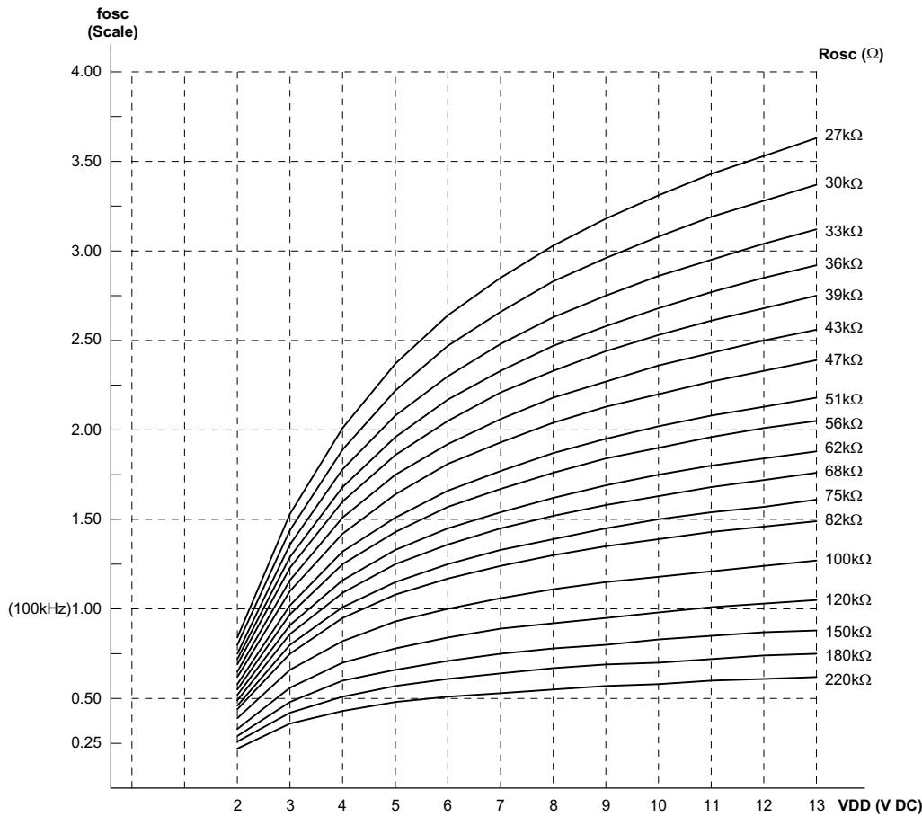
Note: The recommended oscillator frequency is  $f_{OSCD}$  (decoder)  $\geq 50 f_{OSCE}$  (HT12E encoder)
