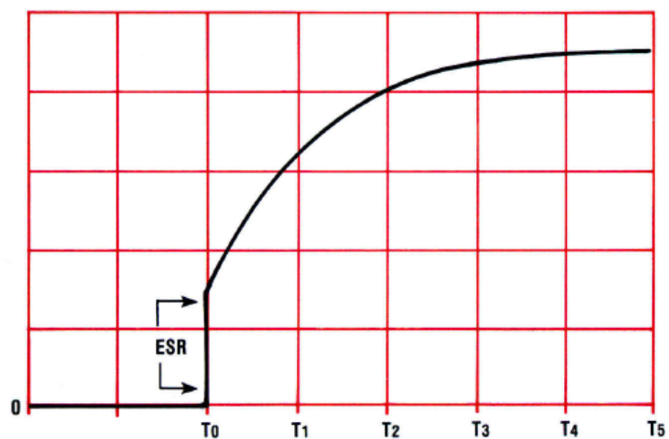
Fig. 7: When there is series resistance, the charging voltage instantly rises to a voltage / \epsilon / (proportional to the resistance in the capacitor and the output impedance of the power supply) before beginning the normal R-C curve.
