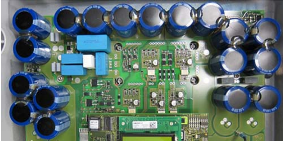
Figure 2.6 The DC-link capacitors in the commercial product ( 300\text{V} , 18 \times 1000\mu F ).
