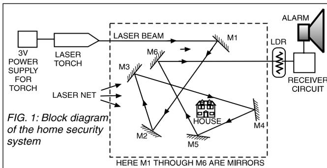
beam by a thief/ trespasser will result into energisation of the alarm. The 3V power-supply circuit is a conventional full-wave rectifier-filter circuit. Any alarm unit that operates on 230V AC can be con-
