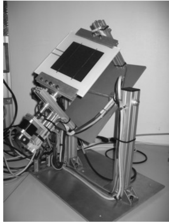
Fig. 7. Prototype built: Electromechanical structure
