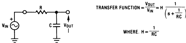
Fig. 4-7. The RC Low-Pass Filter Transfer-Function
