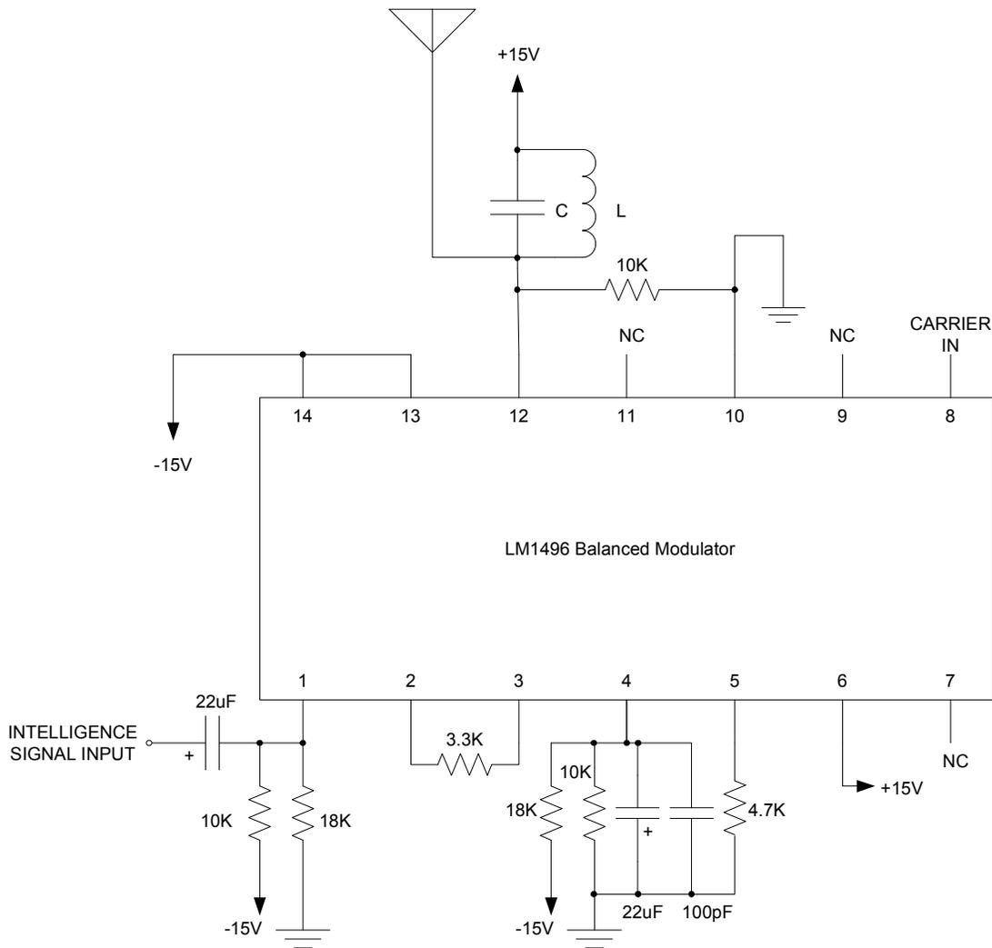
The L and C used in the LM1496 circuit must match the L and C chosen for the Colpitts oscillator which determined the  $f_c$ . Once this circuit is ready, execute the following:
