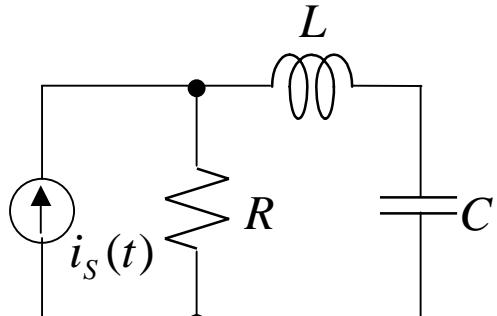
**Step 0:** Transform the circuit into the s domain using current sources to represent capacitor and inductor initial conditions
