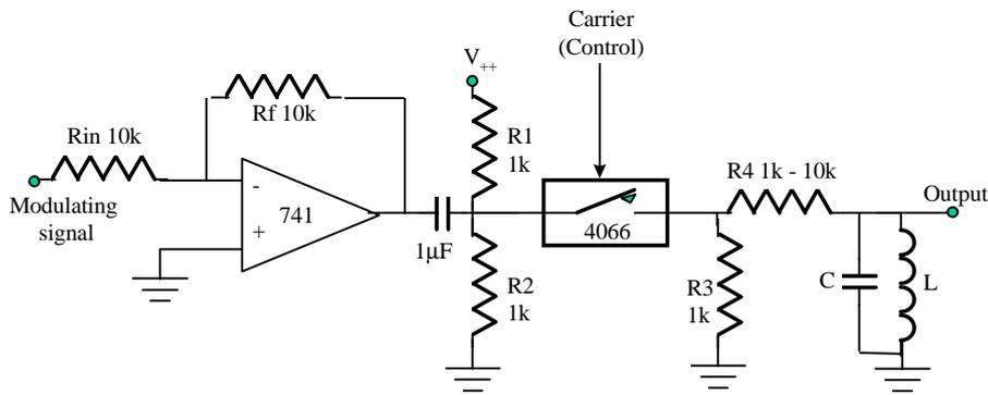
1. The circuit to produce an AM modulator is shown. **Build this circuit, but leaving out the op-amp at this stage - you can add it in when the rest of the circuit is**
