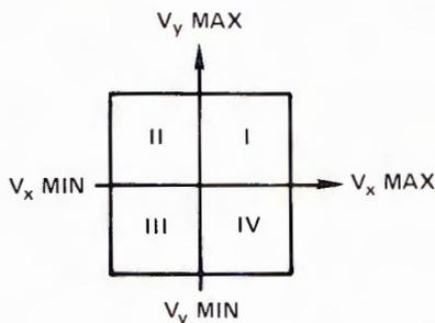
Figure 6. Input plane showing multiplication quadrants
