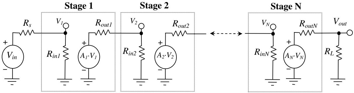
$$A_v = \frac{V_{out}}{V_{in}} = \left( \frac{R_{in(1)}}{R_s + R_{in(1)}} \right) \cdot \left( \prod_{j=1}^{N-1} \frac{A_j \cdot R_{in(j+1)}}{R_{out(j)} + R_{in(j+1)}} \right) \cdot \left( \frac{A_N \cdot R_L}{R_{out(N)} + R_L} \right)$$
