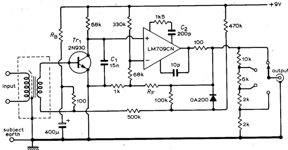
Fig. 1. The circuit of the muscle voltage amplifier.
