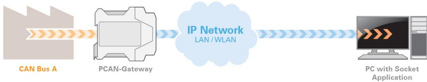
Figure 3: Connection via a Socket application
