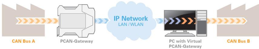
Figure 2: Connection via the software Virtual PCAN-Gateway
