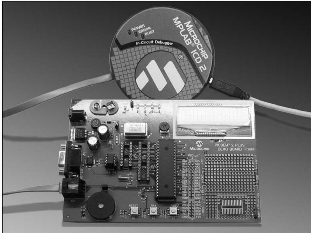
Configure the PICDEM 2 Plus Demonstration Board for the desired oscillator as described in Table 2-1. Refer to the ICE/ICD user's guide for any oscillator configuration requirements.
