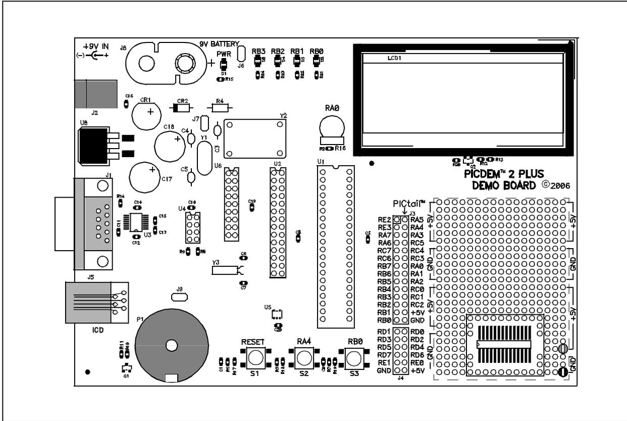
**FIGURE A-2: PICDEM™ 2 PLUS DEMONSTRATION BOARD SCHEMATIC, SHEET 1 (MICROCONTROLLER SOCKETS, LCD OPTIONS, OSCILLATOR OPTIONS, EEPROM AND SENSOR)**
