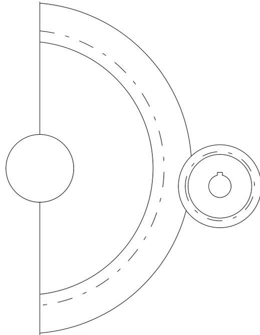
Large gear rotates with shaft. Pot is attached to small gear.
