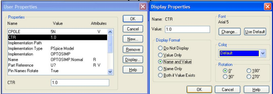
Now that the symbol is all finished, and the two parameters are shown, with their default values. When placed in a schematic for simulation, the user can easily edit the CTR and Cpole as they wish. Save and close the library, but leave Capture open.
