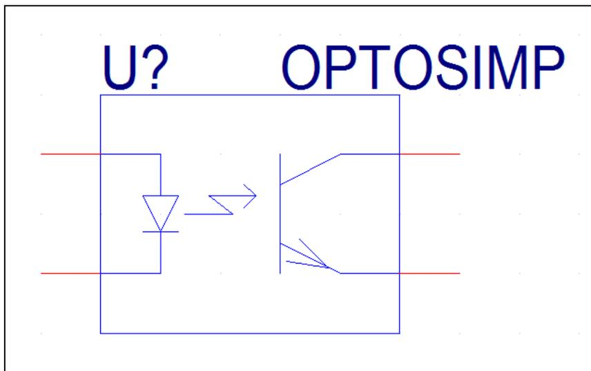
Go to 'Options > Part Properties', and highlight the two parameters. Click 'Display', and select 'Name and Value' and OK. In the User Properties box, a 'V' gets placed in their attributes column indicated that that property are now visible.
