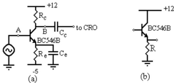
B. Circuit (b) is to be inserted in series at point B to buffer the load capacitance. Calculate  $R$  to give a collector current of about  $1.2 \text{ mA}$ . Assuming a 'typical' value for  $h_{fe}$ , recalculate  $f_H$ . Is the pole frequency introduced by  $C_c$  significantly affected?
