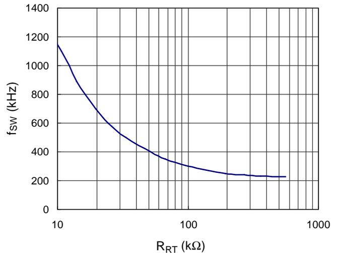
Figure 1. RT vs. fsw at Low Frequency
