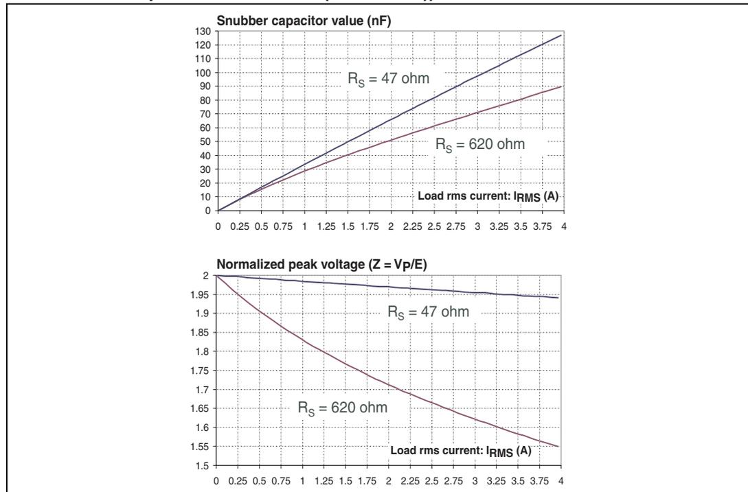
*Note: For inductive load with rms current higher than 4 A, Snubberless TRIACs are recommended.*
