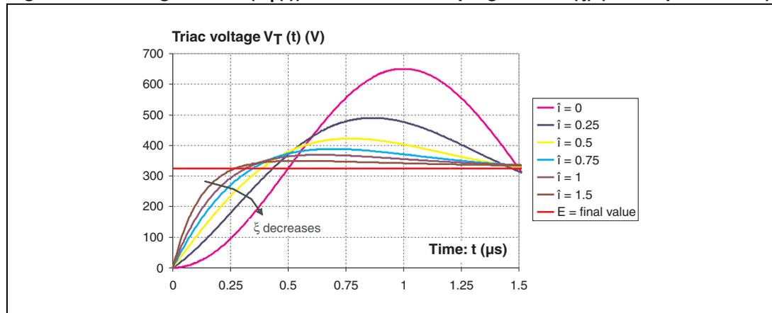
When  $\xi$  is lower than 0.5, the voltage shape is not exponential and the maximum instantaneous slope of voltage rise occurs at a time later than  $t = 0$ .
