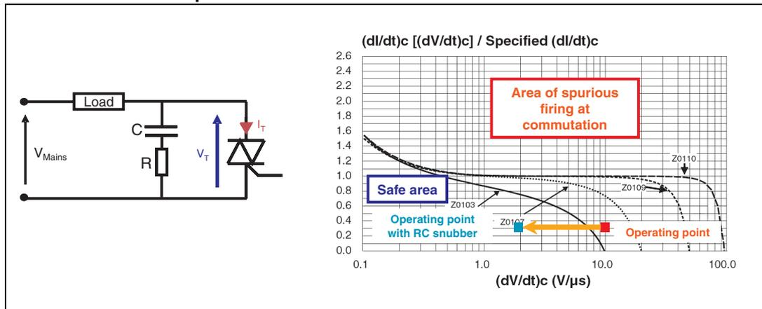
An RC snubber circuit must be used when there is a risk of TRIAC spurious triggering, i.e. when the  $di/dt_{OFF} - dV/dt_{OFF}$  couple, measured in the application, is higher than the TRIAC datasheet values,  $(di/dt)_c$  at a given  $(dV/dt)_c$ .
