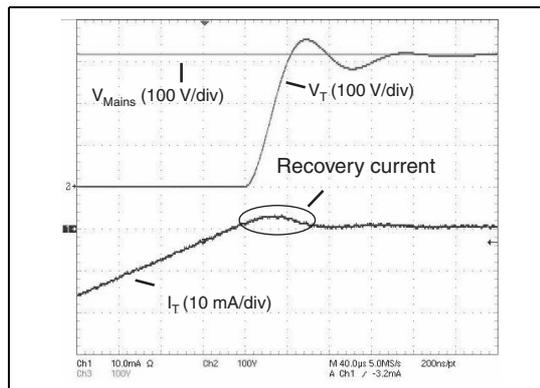
**Figure 2. TRIAC turn-off on inductive load - spurious triggering**
