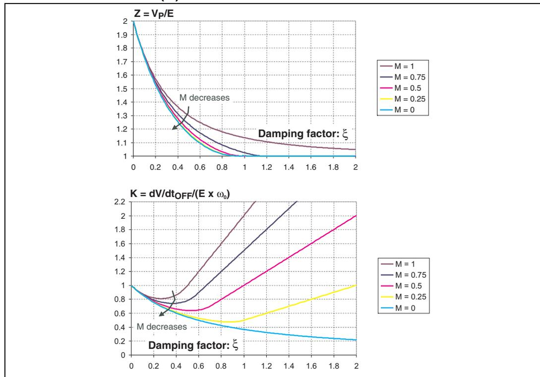
As shown on these two diagrams, the load resistance ( $R$ ) helps to reduce  $dV/dt_{OFF}$  and  $V_P$ . The load impact is significant if the damping factor is higher than 0.2.
