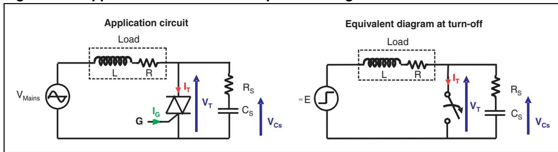
For a second order linear differential equation with a step function input, the voltage variation across the snubber capacitance ( $V_{C_S}(t)$ ) and the TRIAC ( $V_T(t)$ ) is given by:
