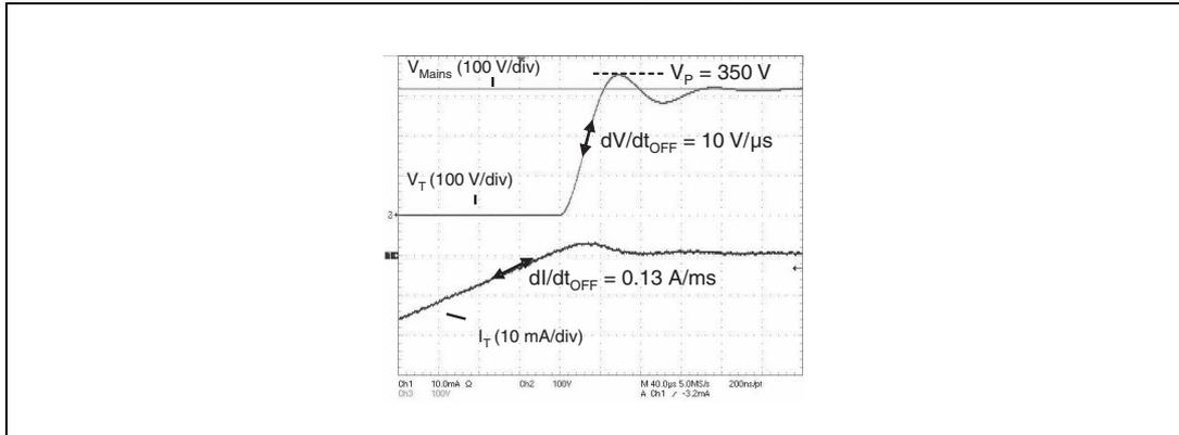
An RC snubber circuit must be used when there is a risk of TRIAC spurious triggering, i.e. when the measured  $dI/dt_{OFF}$  and  $dV/dt_{OFF}$  values are higher than the specified  $(dI/dt)_c$  and  $(dV/dt)_c$  values.
