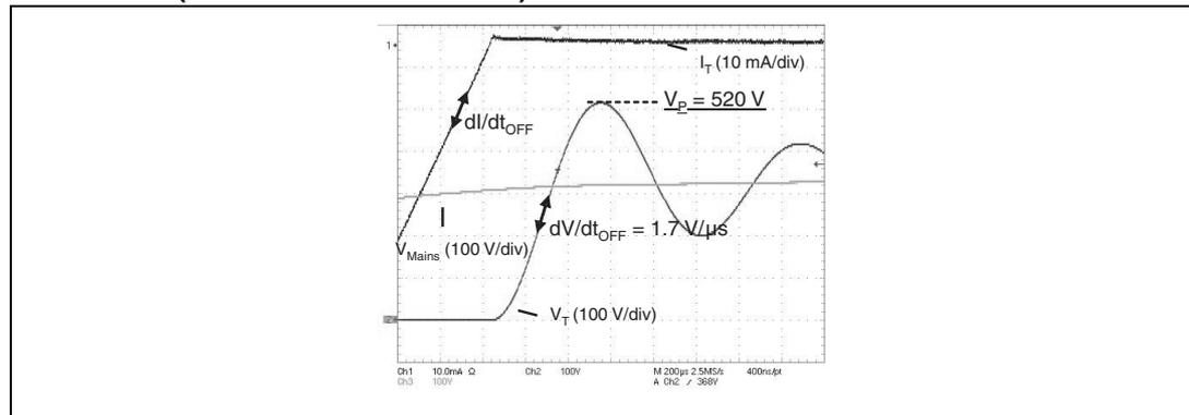
The second method of RC snubber circuit design allows a quicker snubber capacitor choice. The capacitor is directly chosen from the load rms current (refer to *Figure 12*). Pure inductive loads are considered and the slope of the reapplied voltage is fixed to 2 V/μs.
