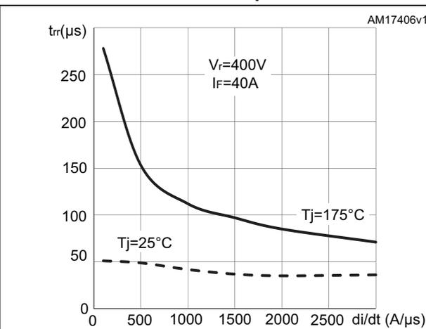
Figure 33. Reverse recovery charge vs. diode current slope
