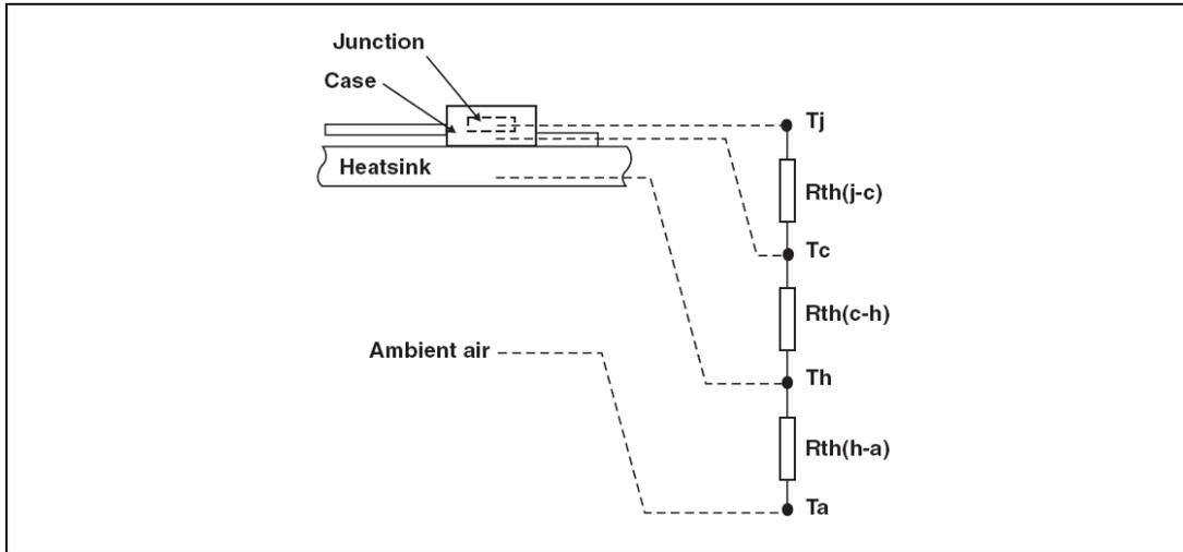
The thermal resistance stated in datasheet refers to the above mentioned  $R_{TH(J-C)}$  and to the overall  $R_{TH(J-A)}$ .
