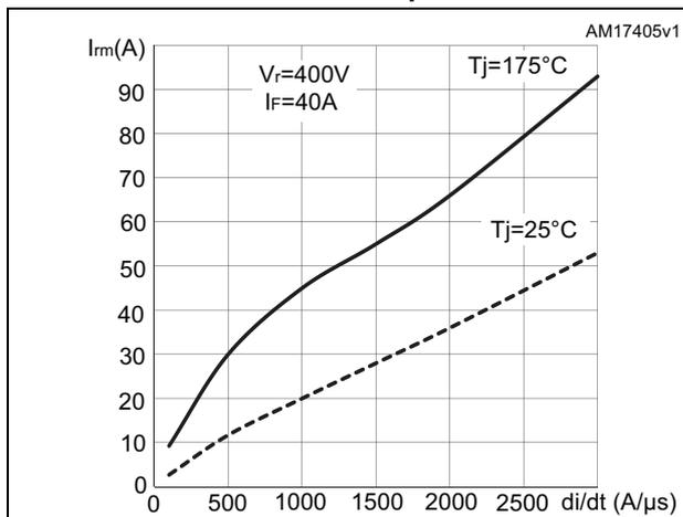
Figure 32. Reverse recovery time vs. diode current slope
