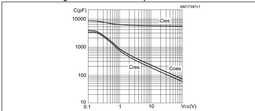
Figure 19 shows a graph of typical capacitance values versus collector-to-emitter voltage.
