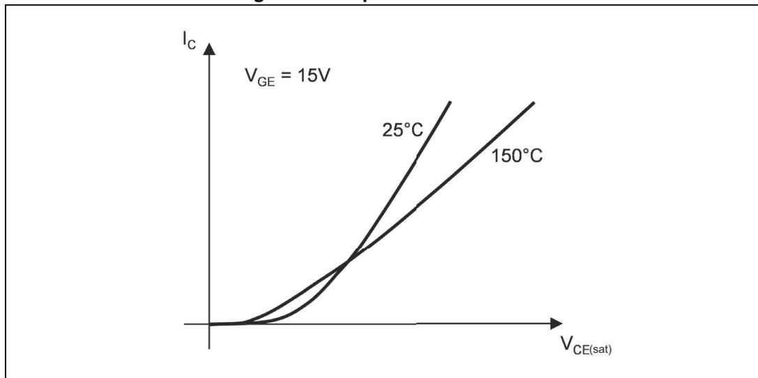
If crossover point is well below  $I_C$  operation range (like the STGW40V60DF), the IGBT has a positive temperature coefficient.
