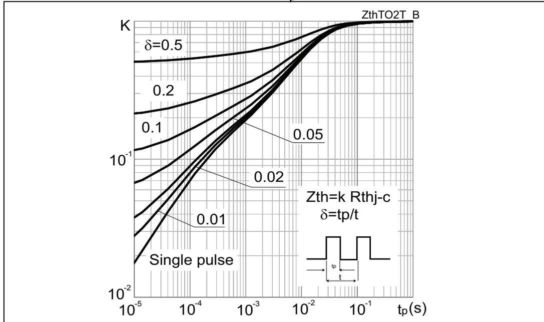
Figure 13 shows the variation of the normalized thermal impedance for the specified pulse duty factor  $\delta=tp/t$  as a function of the loading time  $t_p$  (pulse width).
