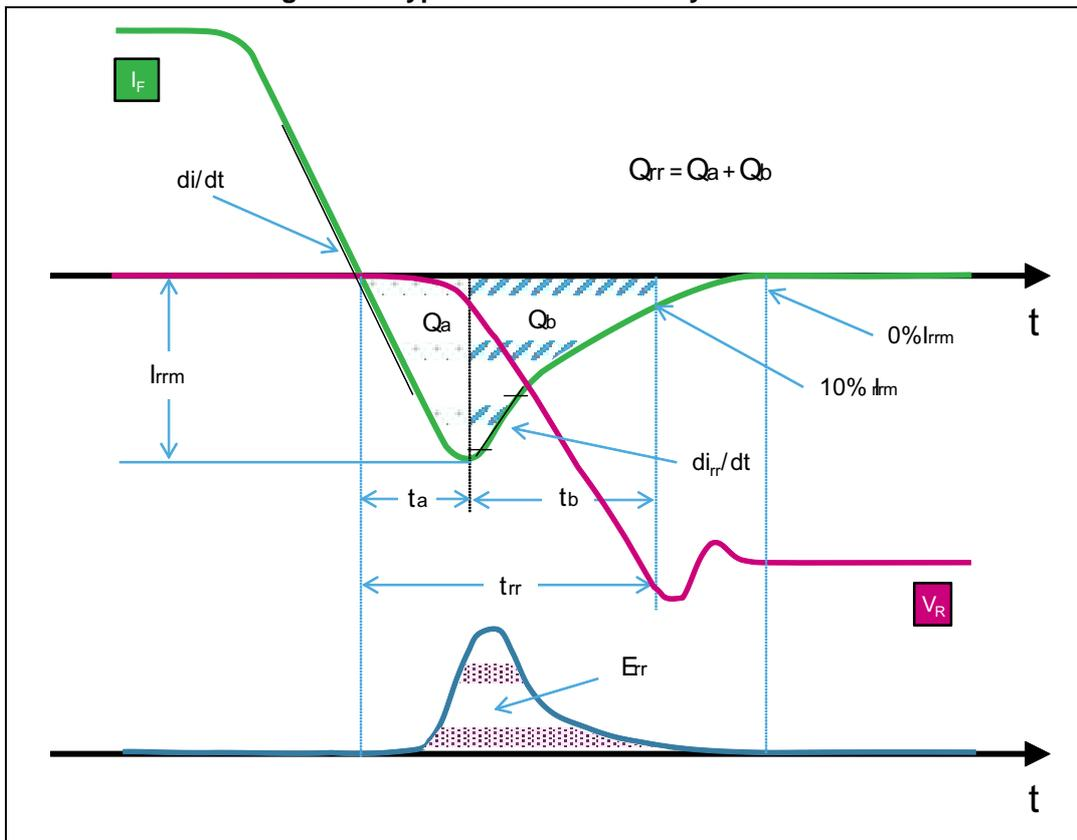
Figure 31. Reverse recovery current vs. diode current slope
