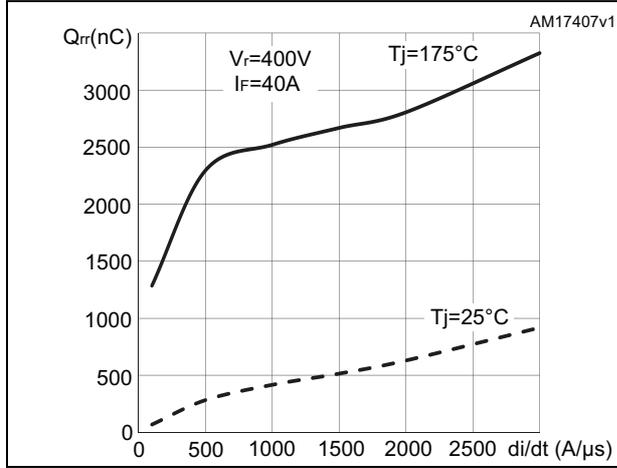
Figure 34. Reverse recovery energy vs. diode current slope
