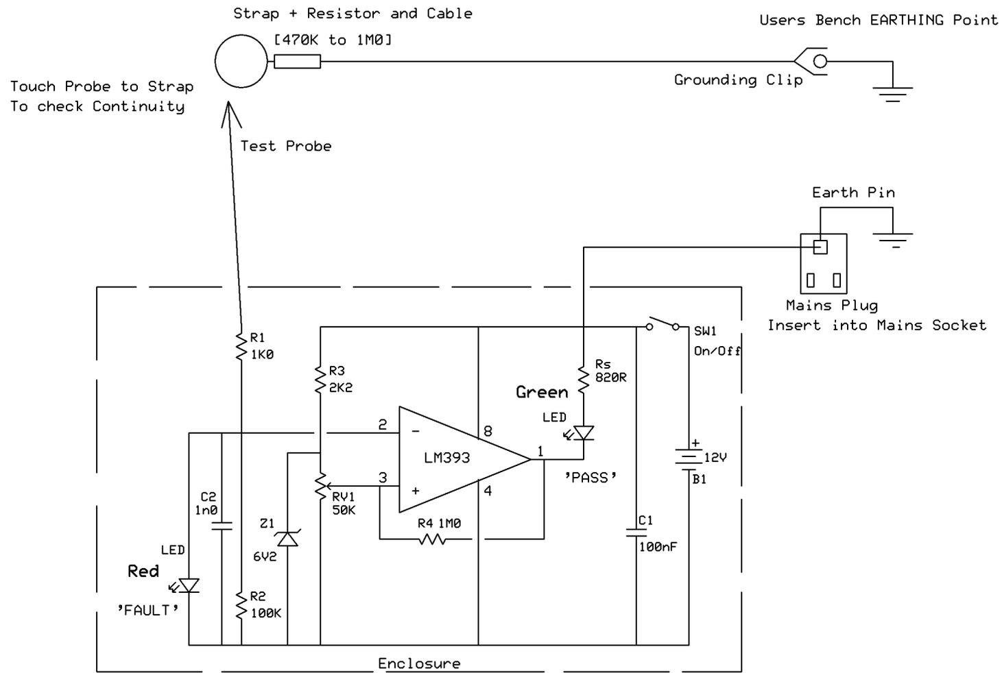
'FAULT' LED will light if Strap Resistor is missing
