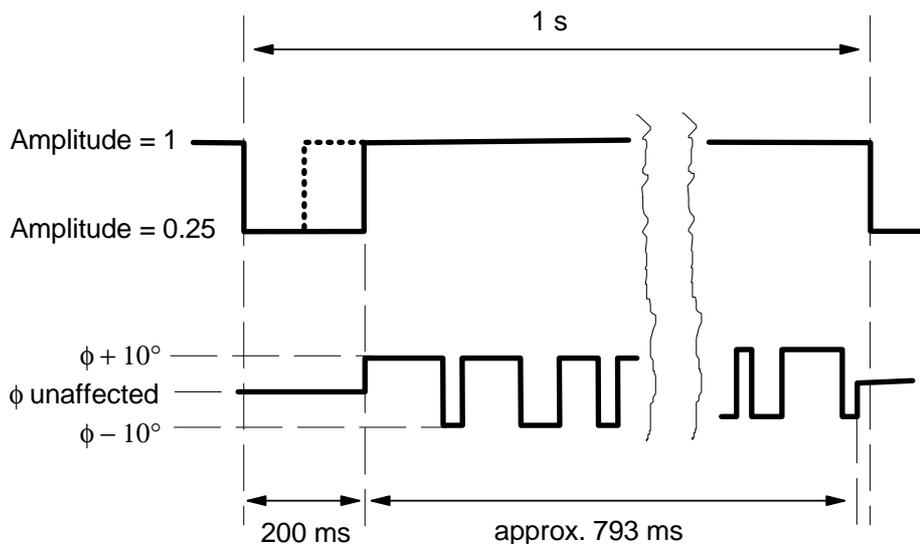
Figure 1b. The 512 step pseudorandom sequence starts 200 ms after the full second, defined by the falling edge of the amplitude, and ends about 7 ms before the next second. This ensures that the falling edge is not disturbed. The transmitter phase is shifted by  $\pm 10$  degrees. Note: Timing in this sketch is not to scale.
