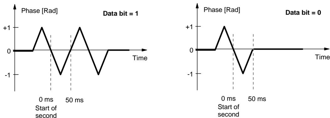
Figure 2. Phase shift keying of France Inter on 162 kHz. The rise and fall time of 1 Rad / 25 ms corresponds to a frequency shift of  $\pm 6$  Hz, which is inaudible in the audio broadcast signal. There are either one or two cycles of 100 ms at the begin of each second (except second 59), depending on whether a logical "0" or a "1" is transmitted.
