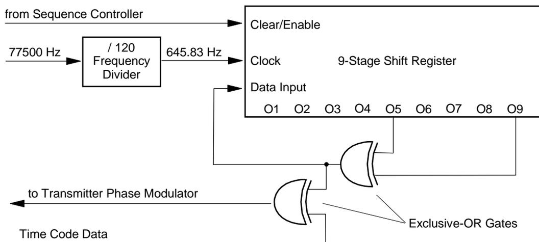
Figure 1a. A pseudo random sequence of 512 steps is generated by means of a feedback shift register. Not shown is a mechanism to force the shift register out of the “all zero state” at the beginning of the sequence. Sequence inversion keying is used: The phase shift is inverted if a logical “1” is transmitted.
