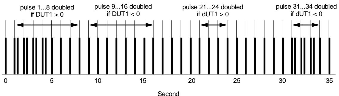
Figure 5. Coding of the deviation between astronomical time UT1 and atomic time UTC. The difference in seconds is given by  $0.1 \times \text{DUT1} + 0.02 \times \text{dUT1}$ . In this example, DUT1 is +4 and dUT1 is -3, hence  $\text{UT1} - \text{UTC} = +0.34$  seconds.
