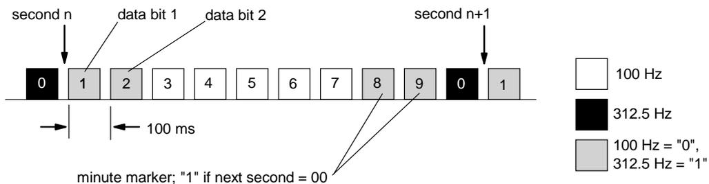
Figure 4b. Relationship between subcarrier frequencies and data
