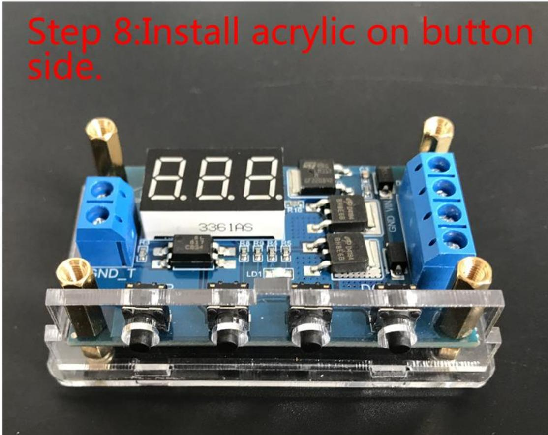
Step 9: Install acrylic. Note the corresponding point
