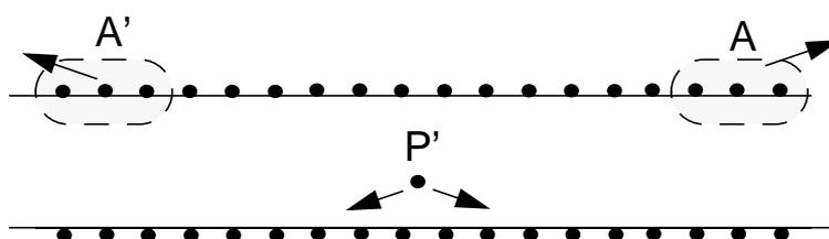
Fig. 6: Influence of a Constant Surface Charge (for Points P' off Axis)
