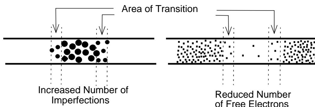
Fig. 13: Different Mechanisms for Electric Resistance
