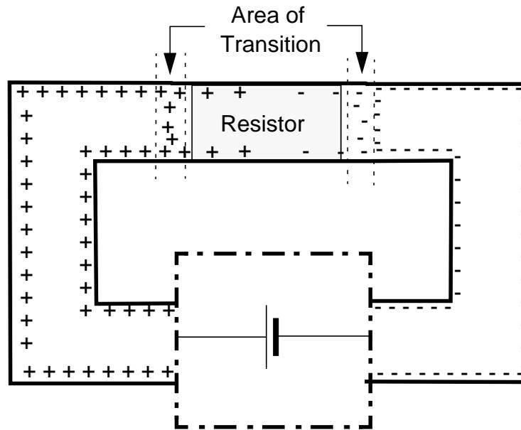
Fig. 14: Surface Charge Distribution (Circuit with one Resistor)
