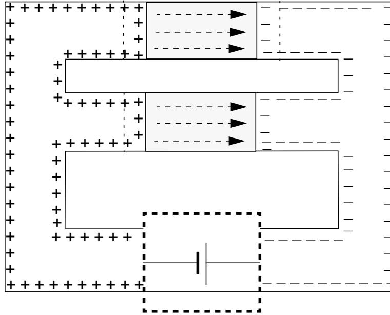
Fig. 16: Surface Charge Distribution in a Parallel Circuit
