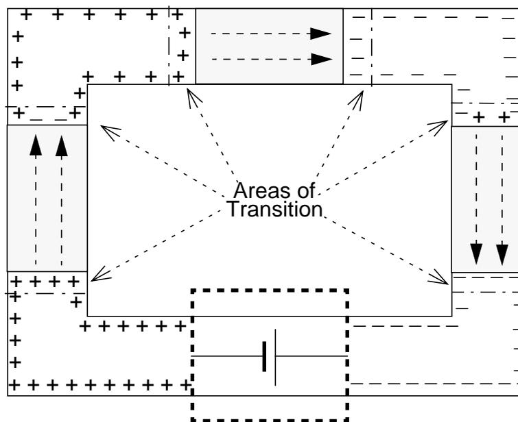
Fig. 15: Surface Charge Distribution in a Series Circuit
