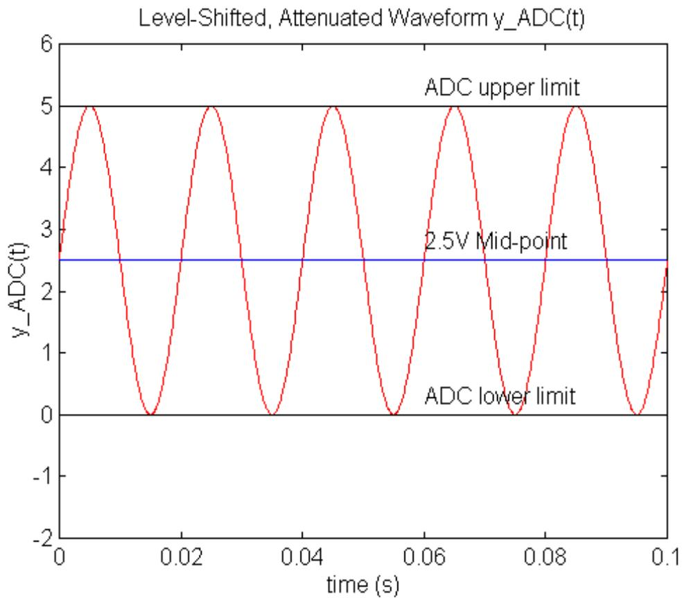
The aim of the task is to design and implement the circuitry that effectively performs the mathematical operation:-
