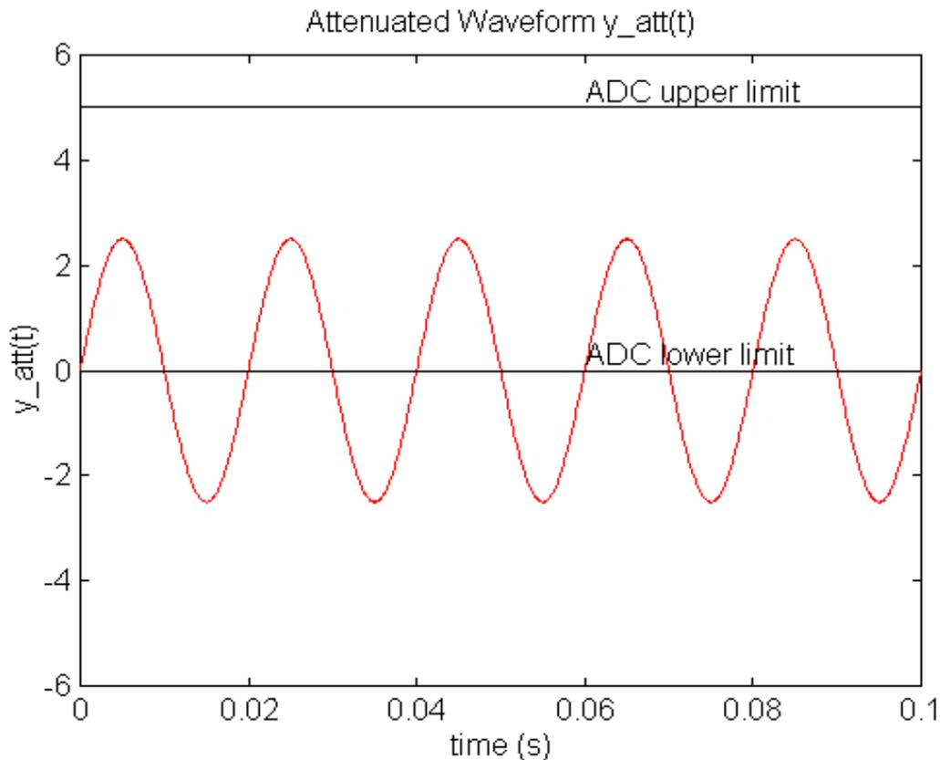
This is certainly an improvement as the positive-going cycle of the waveform can now be sampled in its entirety by the ADC. However, the ADC will still not be able to sample the negative-going cycle of the waveform.
