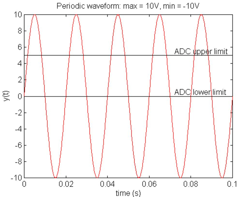
Now the ADC can sample signals ranging from 0V to 5V. This presents us with two problems:-
