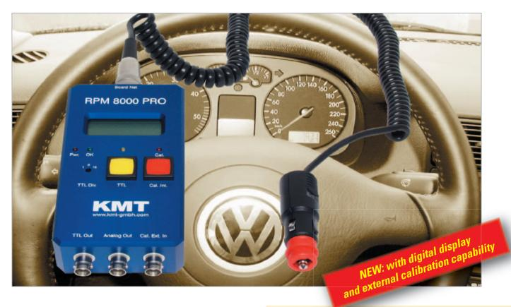
PM-8000-PRO offers a discerning solution for automotive RPM measurement without an additional sensor: the instrument is simply connected via a standard jack to the cigarette lighter socket and the engine speed is shown directly on the LCD display, or is available as a proportional analog voltage or frequency for recording purposes.
