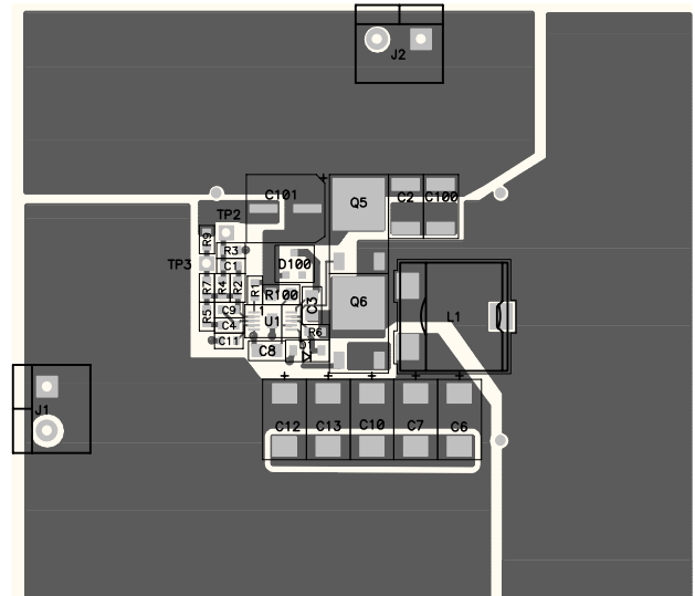
Fig. 34. Massive copper pours help spread heat.
