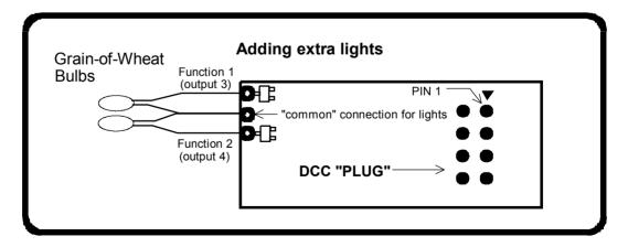
**Function output ratings:** Due to the high in-rush current of incandescent grain-of-wheat type bulbs (about 10 times their normal operating current) function outputs are rated at 40mA each if used with incandescent bulbs. We recommend the Miniatronics part number mentioned above. If you wish to use 50-100mA rated lamps we recommend a 22 ohm 1/4 Watt series resistor in function leads with each bulb (this will also greatly extend bulb life).
