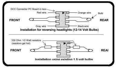
**Recommended Lighting**: If you use LEDs we recommend a 1K ohm 1/4 Watt series resistor in each function lead.
