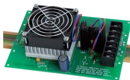
PAD127 mounted in evaluation kit
