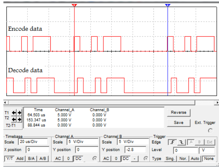
Fig. 9. The required time for sending 8 bits of data (88.844μs / 90kbps), and the ability of the receiver to decode these encoded data at this speed
